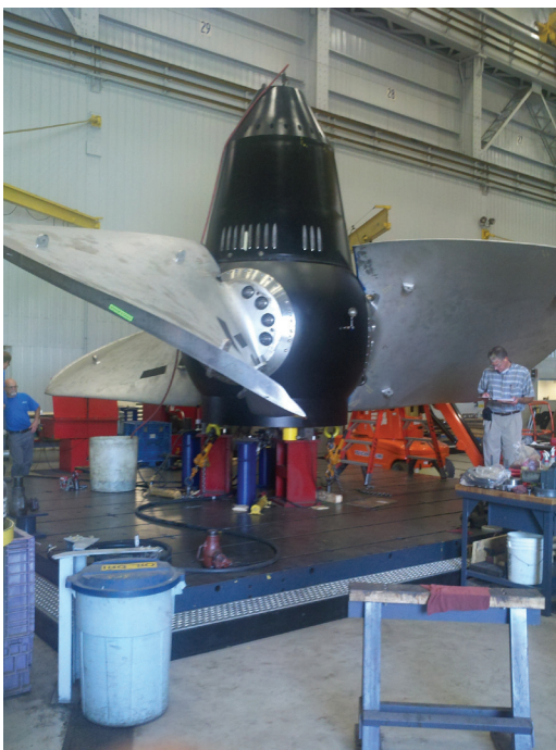
Crew members, along with MWH staff, perform assembled runner tests on the Cannelton Unit 1 Turbine Runner in York, Pennsylvania, to examine the movement of the blades.
